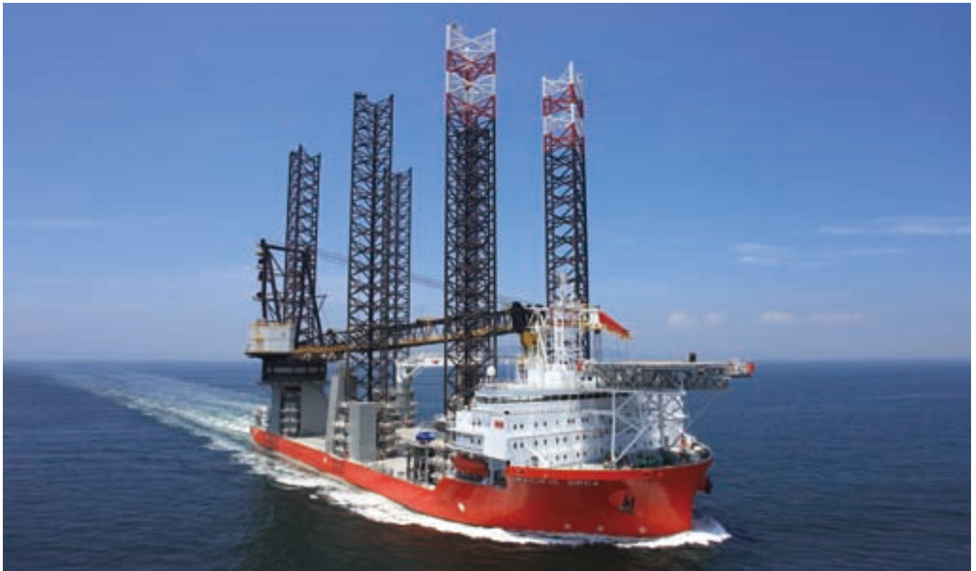
Pacific Orca , the world's largest wind farm installation vessel, was the first of two wind farm installation vessels delivered to SPO in 2012.
