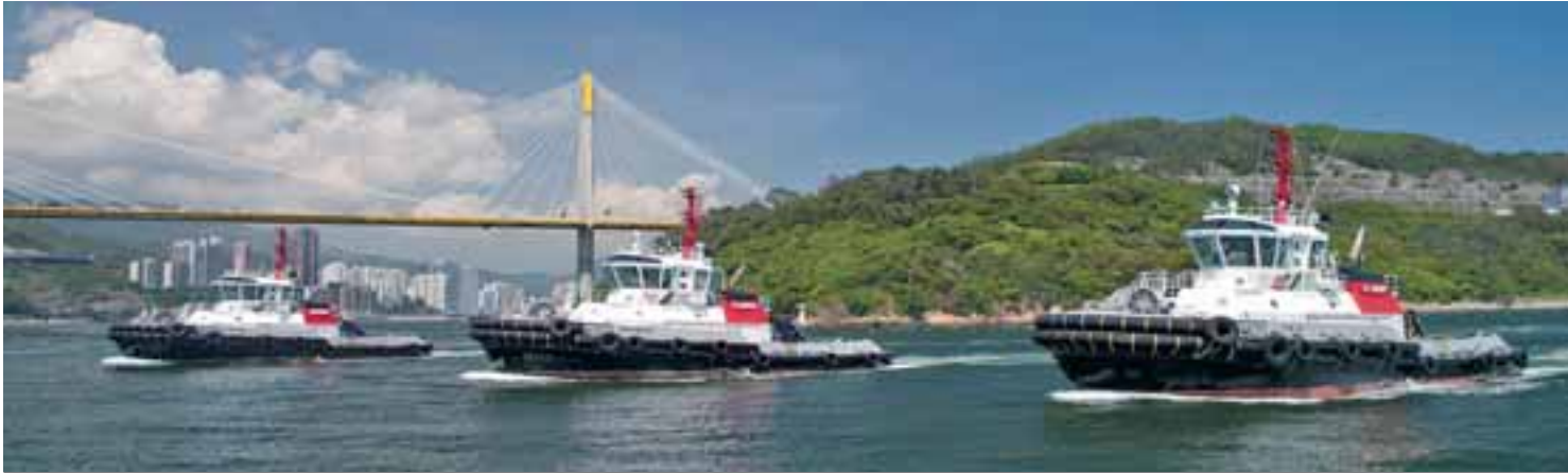
HUD took delivery of the final two (of an order of four) 5,000 bhp tugs in 2012. They are the biggest tugs ever operated in the port of Hong Kong, providing harbour towage, salvage, fire-fighting and oil-pollution control capabilities.
